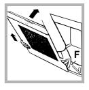
3. Grip the door on the two external sides and close it approximately half way. Unlock the door by pressing on the clamps **F**, then pull the door towards you lifting it out of its seat (*see diagram*). To replace the door, reverse
